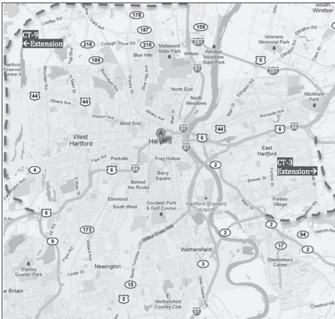
Figure 3: Proposed I-291 and CT-3 extensions fill the remaining two quarter-rings, integrating the metropolitan area while minimizing neighborhood and environmental impact. Extant I-291 and CT-9 (which intersects I-91 just south of this map in Berlin, CT) complete the ring system.
