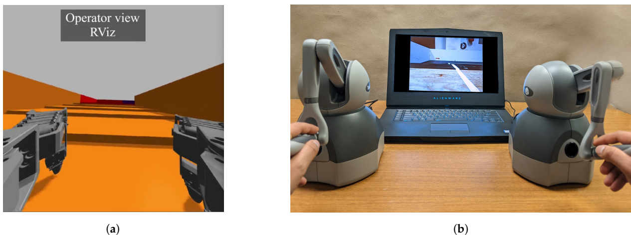
Figure 4. Typical visual feedback received by operator, rendered either from (a) a simulated streaming RGB camera mounted to the robot base or (b) the Raspberry Pi Camera V2 mounted to the physical robot. In both cases, feedback is rendered on a standard LCD display.
