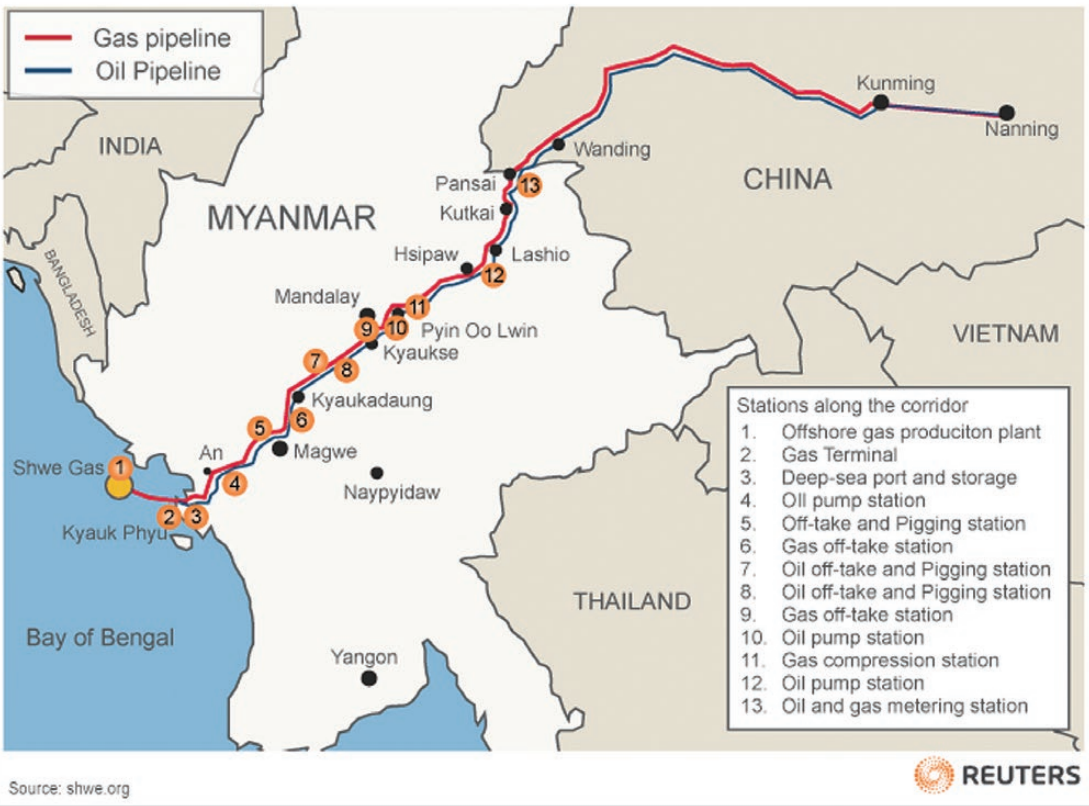
Figure 3. The cross-border China–Myanmar oil and gas pipeline: from Kyaukpyu to Kunming through Ruili.
