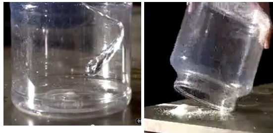
Figure 2: Unexploded Rupert's drop (left) and powder (right) resulting from the explosion following cracking of the tail. (Courtesy of Corning Museum of Glass.)
