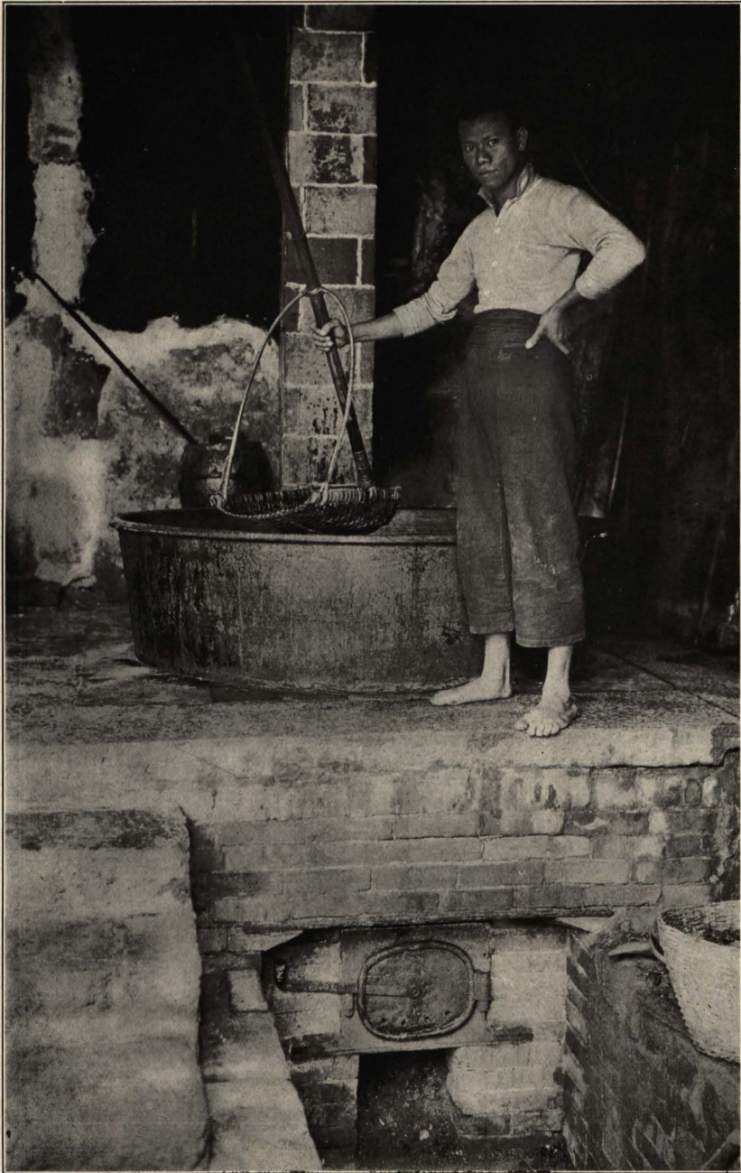
PLATE I. THE IRON PAN IN WHICH THE SOY BEANS ARE BOILED.
